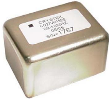
Oven controlled crystal oscillator (OCXO), Crystek CO27VH15DE
